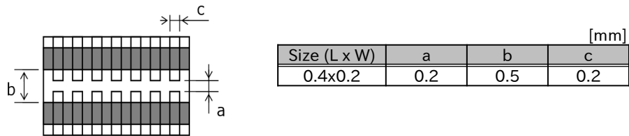
Fig. 2: Board / Test Jig of Adhesive Force of Terminal Electrodes, Vibration, and Thermal Shock
